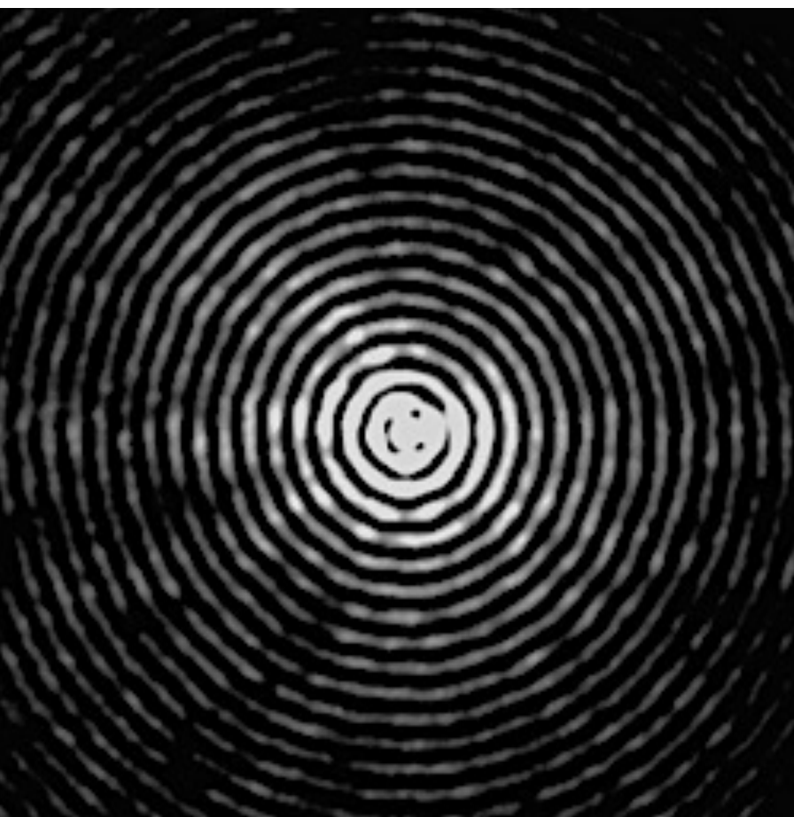
Figure 3: Experimentally observed Point-Spread Function of Bessel beam
